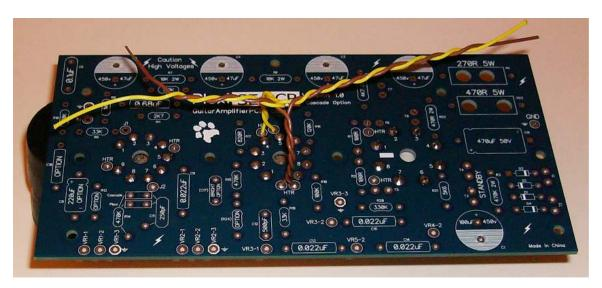
Route the four remaining wire leads to the tube heater (HTR) locations. Trim for length, strip the insulation, and solder in place.
