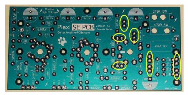
Instead of using spade connectors, the wire leads should be soldered directly to the board in location marked above. Don't worry about this now. It will be cover later when the board is installed in the chassis.
