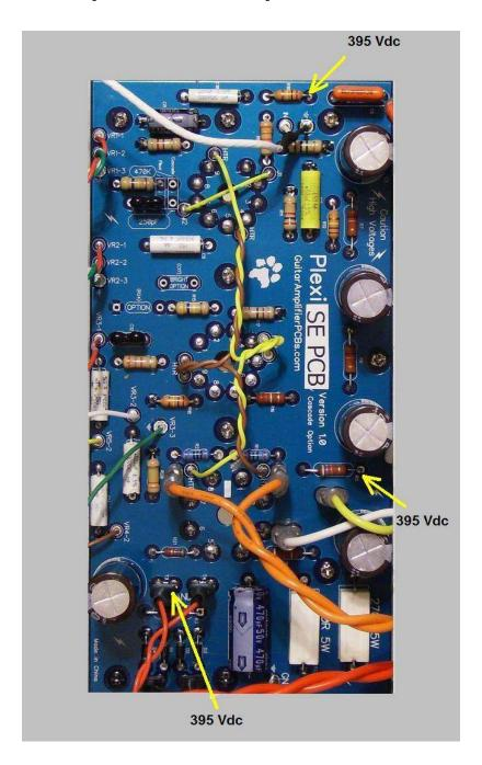
The unloaded B+ voltage should measure the same all the way up the power rail. A slight fluctuation is normal. If a difference greater than 5-10 Vdc is measured, something is drawing current when it shouldn't. Turn off the amp and troubleshoot the problem.
