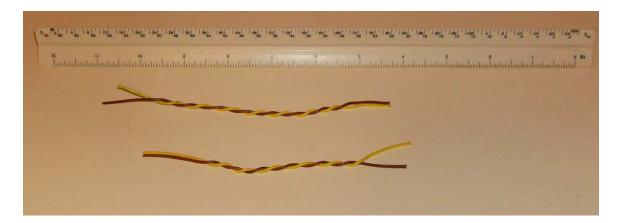
Twist the wires together as shown.
