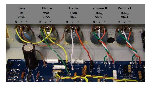
Guide the wires from the circuit board to their respective solder posts on the control potentiometers. Trim the wires to length, strip the insulation from the ends, and solder the wires in to place on the control pots. Refer to the schematic and layout diagram for additional information regarding the wiring hookup locations.
