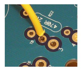
Fasten the ground wires from the Plexi SE PCB and the output transformer to the star ground screw post.
