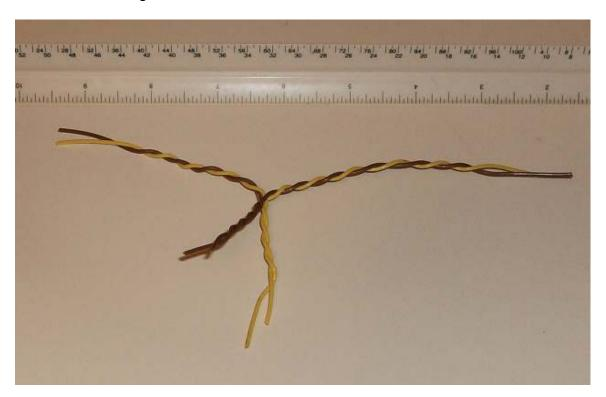
Strip  $\frac{1}{4}$ " of the insulation off of the ends of the wires. Insert the leads into the solder pad locations on the middle tube socket labeled "HTR" for heaters.
