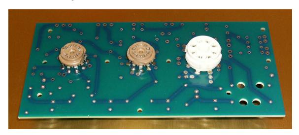
Insert the tube sockets as shown. The noval (9-pin) sockets only go in one way (on the back side). However, the octal (8-pin) socket needs to be properly oriented with the circuit board. Position the notch in this socket so that it is pointing toward the two noval sockets.
