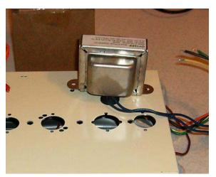
Secure the output transformer to the chassis using the stock fasteners.
