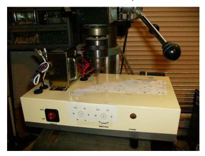
Here, a unibit was used to drill out the 7/8" hole for the two (2) additional tube
