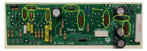
The filtering capacitors are not installed at this time. The height of these capacitors interferes with the installation of the other components. These capacitors will be the last component installed.
