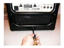
Locate the screw caps on the top of the EVJ. Using a standard screw driver, the smaller the better, pry up the caps until you can pull them out of their sockets.
