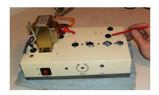
Guide the leads through the grommets and seat the output transformer in place. Position the output transformer with its primary to the front and secondary to the back as shown.
