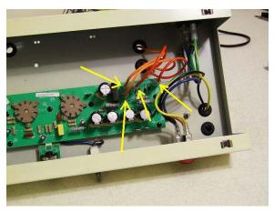
Remove the six (6) screws fastening the circuit board to the chassis.
