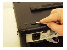
Remove the four chassis screws and pull out the chassis.
