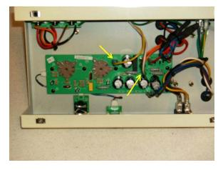
Pull these two spade connectors from the main circuit board.
