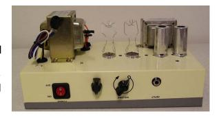
Make sure the screws used to mount the tube hardware do not contact the circuit board or any component on the inside of the chassis.
