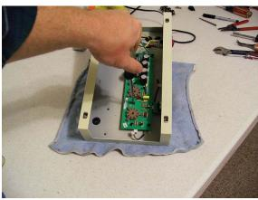
Remove the stock circuit board and pull all of the power transformer leads to the rim of the chassis.
