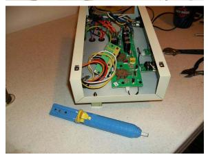
Now that all of the leads are free, remove the mounting screws to separate the transformer from the chassis.
